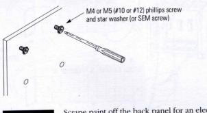
Scrape paint off the back panel for an electrical connection between the chassis and back panel.
