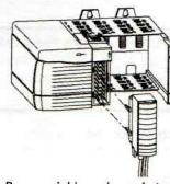
3. Press quickly and evenly to seat the RTB on the module until the latches snap into place.
